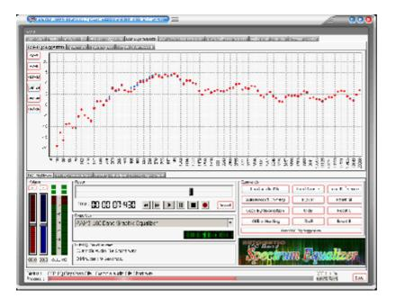
The DSP-EQ Graphic Equalizer Processor is used for processing the adjusted sound and can only be adjusted from -12dB to 12dB per EQ band. So in the real world (hearing audio) the lowest possible cutoff is -12dB by the DSP-EQ Equalizer. The highest possible boost per EQ band is 12dB. So even when you use the Spectrum Reference Adjust Charts and DSP-EQ Adjust charts, the possible boost can only be between -12dB and 12dB on the outcome of the DSP-EQ Graphic Equalizer Processor.
